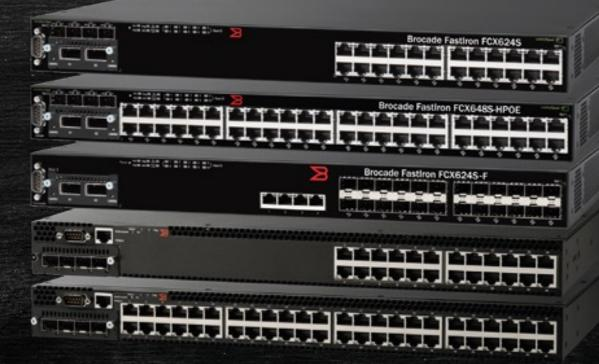
A switch is more intelligent than an Ethernet hub, which simply retransmits packets out of every port of the hub except the port on which the packet was received, unable to distinguish different recipients, and achieving an overall lower network efficiency.
